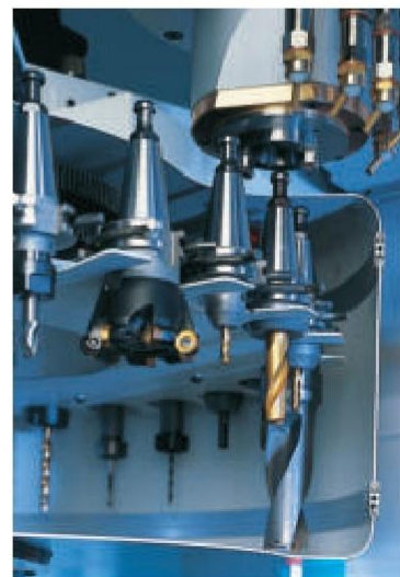
The compact pick-up changer comfortably fits 24 tools.
