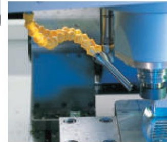
Coolant system with auxiliary tank. To keep the coolant temperature low even with high production output, an additional tank with 600 litre capacity is used. Consistent coolant quality is ensured through automatically actuated circulation system after two hours of inactivity. A high pressure pump (40 or 80 bar) allows the use of internally cooled tools.
