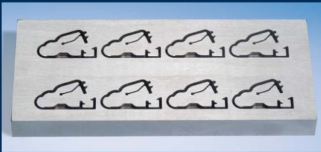
Multi-cavity-machining with 8 cavities
